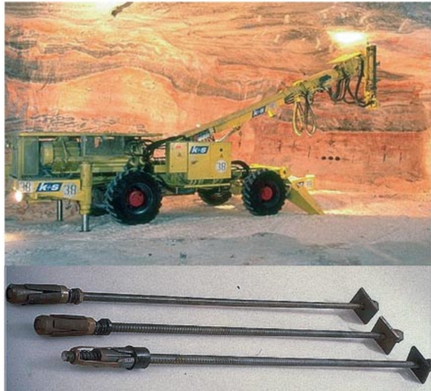
Abb. 1: Firstankerbohrwagen / Roof bolter and rockbolts
