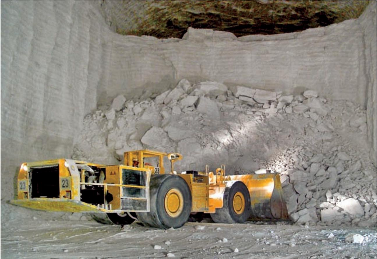
Abb. 3: Fahrlader in Kammer / Scoop in a stope
