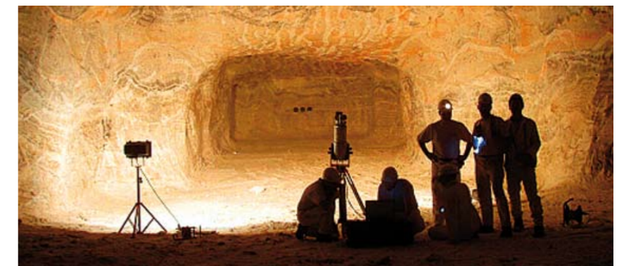
Abb. 5: Scannen eines Bohrortes / Profiling of drilling site
