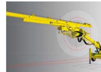
Abb. 4: Kollisionsmodell des Bohrwagens / Model of drilling jumbo
