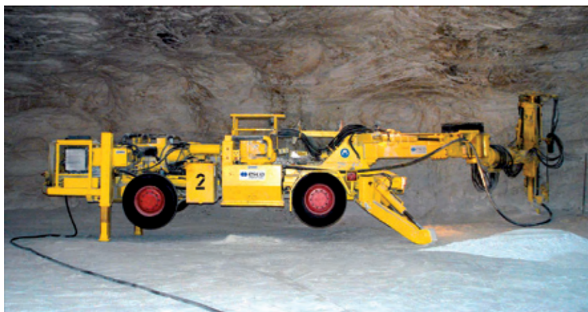
Abb. 6: Strossenbohrwagen SMAG BW 50 S 1 | Bench drilling jumbo – SMAG BW 50 S 1
