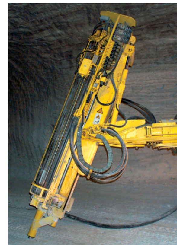
Abb. 7: Lafette des BW 50 S 1 in Bohrstellung | Carriage of BW 50 S 1 in drilling position
