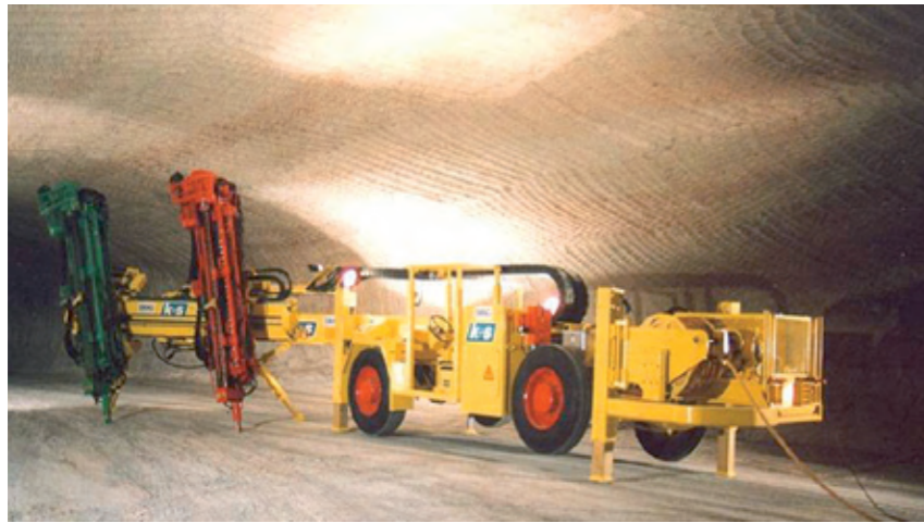
Abb. 5: Strossenbohrwagen SMAG BW 50 S 2 | Bench drilling jumbo – SMAG BW 50 S 2
