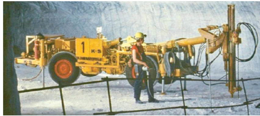
Abb. 3: Strossenbohrwagen SMAG BW 41 / Bench drilling jumbo – SMAG BW 41
