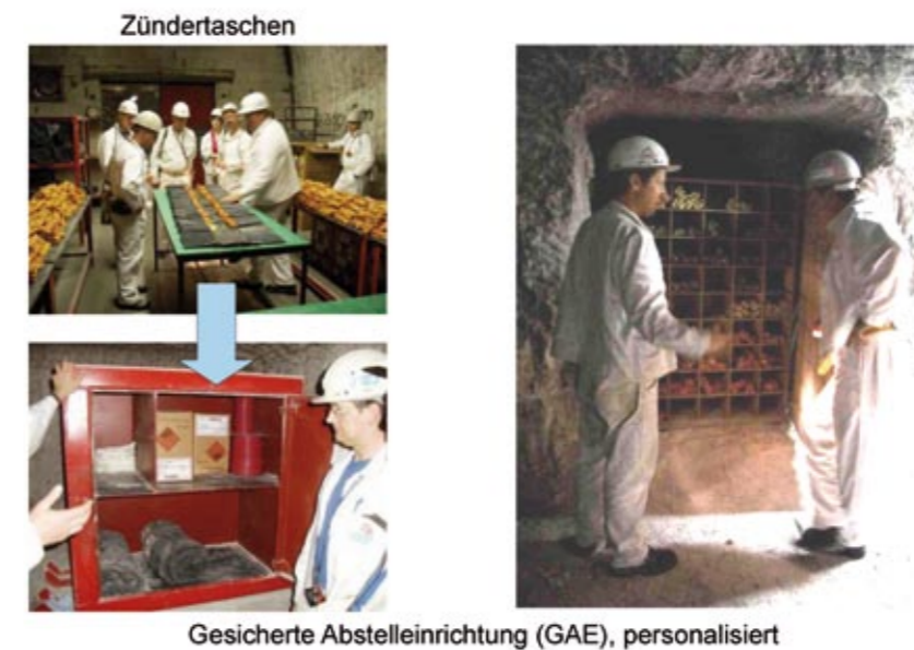
Abb. 6: Sprengmittellogistik unter Tage – Sprengzünder Variante 2/Underground Explosives Logistics – Detonators Variant 2
