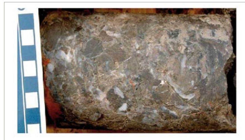
Fig. 7: Dolomite breccia. Well 043-A27: 295.40–295.55 m (scale bar in centimeters) | Dolomitbrekzie. Bohrung 043-A27: 295,40–295,55 m (Maßstab in Zentimetern)
