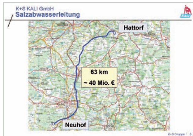
Abb. 8: Salt Water Pipeline
