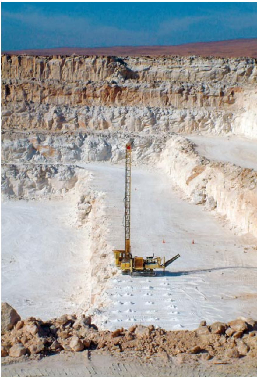
Abb. 8: Sprengloch-Bohranlage beim Abbohren einer Strosse. Foto: SPL / Blast-hole drilling machine during drilling of a bench. Photo: SPL
