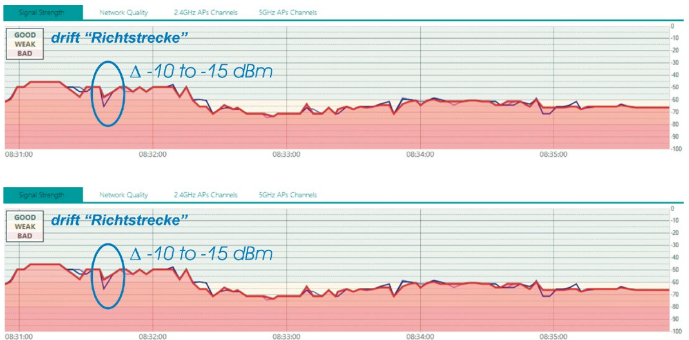
Figure 3: Fluctuation in signal strength at the site “Wlhm-Std.-S”31
